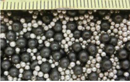
Figure 2. Photograph of the bi-disperse mixture of glass beads.
