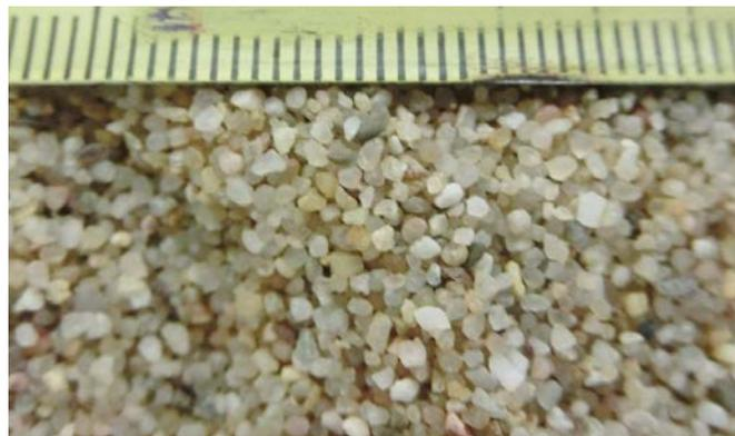
Figure 4.16: Photograph of material M2, coarse sand
