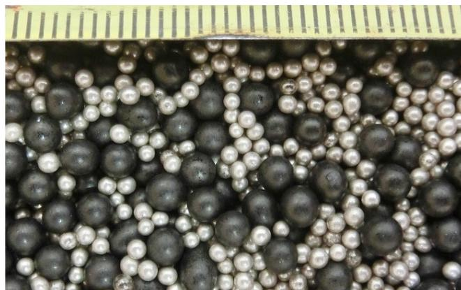
Figure 4.17: Photograph of material M3, glass beads mixture
