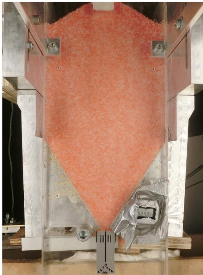
Figure 4.9: Photograph of model silo showing stopwatch and grid points
